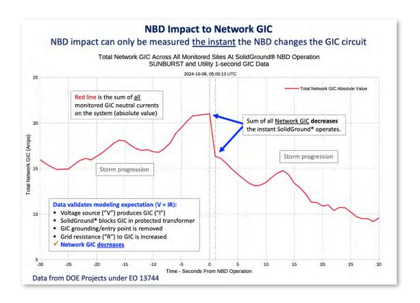
DOE's data consistently shows that **blocking GIC** in the neutral of transformers <u>decreases Network</u> <u>GIC</u>. (i.e. GIC is <u>not</u> being re-directed everywhere else, grid resilience is improving). The more NBDs installed on the power grid, the more resilient the power grid becomes allowing the grid to operate through severe GIC events. **Modeling assumptions need to be updated to reflect the data.**
