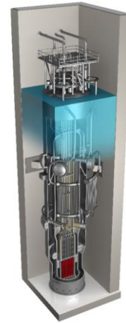
Figure 24. NuScale Power Module (courtesy of NuScale)
