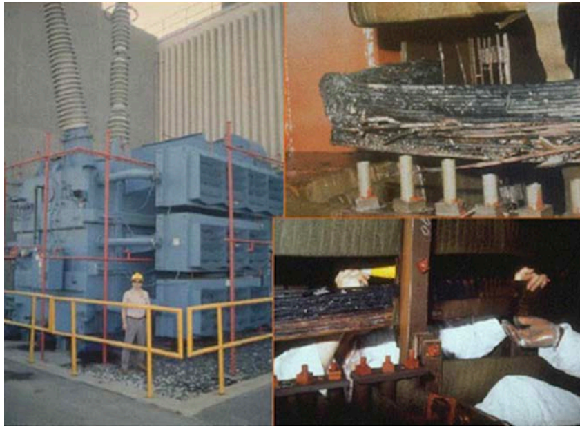
March 1989 magnetic storm damage to a high-voltage transformer at a nuclear power center in Salem, New Jersey. Photo credit: Dr. Jeffrey J. Love, USGS
