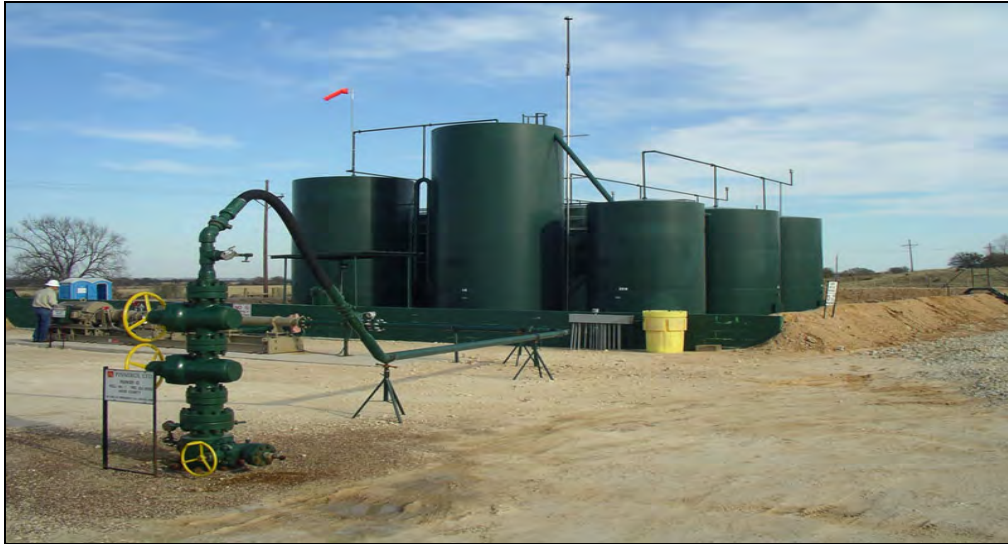
Figure 13 - Typical wellhead in Warm Climate. (GTI) No methanol or other injection equipment for freeze mitigation. Flow line is elevated without insulation of other protection from cold weather. Tank battery and other production equipment are not protected from cold weather. (Ref. 4)
