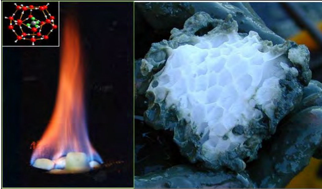
Figure 14 – Hydrate Photos – Inset is the Water- Methane Hydrate Structure (Ref. 16, 17) (Photo Credits National Energy Technology Center (DOE) and Wikimedia Commons)
