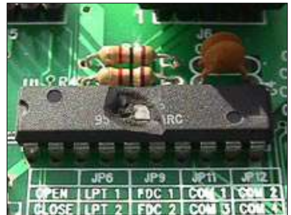
Figure 2 - Integrated Circuit Damage Caused by an RFW
