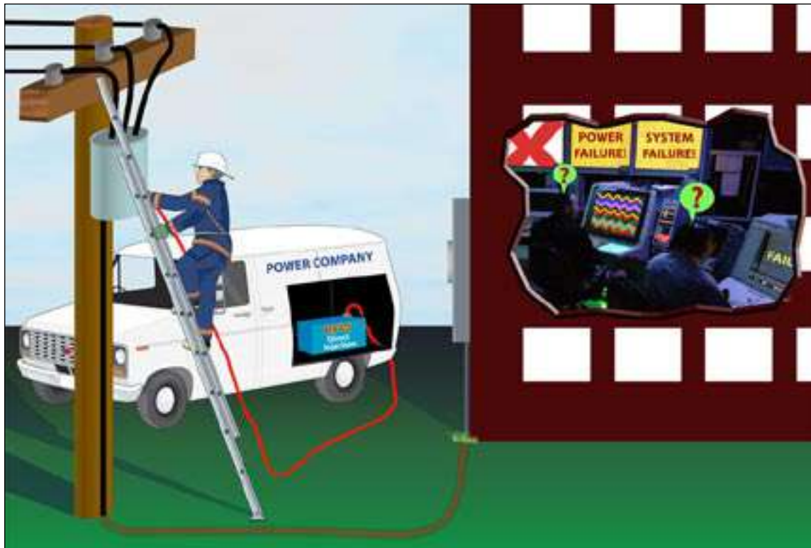
Figure 6 - Illustration of Conducted Threat from an RFW
