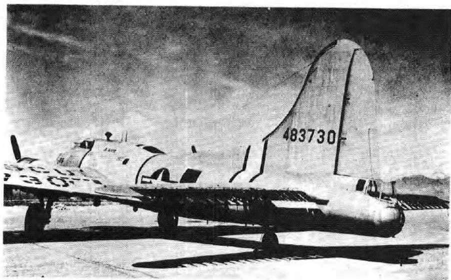
Figure 5.95b. Aircraft after tail exposed to a nuclear explosion (2.4 psi peak overpressure).
