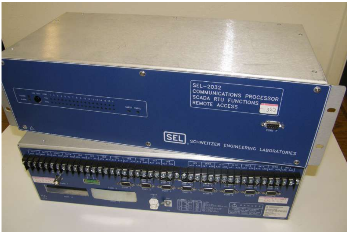
Figure 7-12. Modern SCADA unit. This is the SEL-2032 (front view on top, back view on the bottom).
