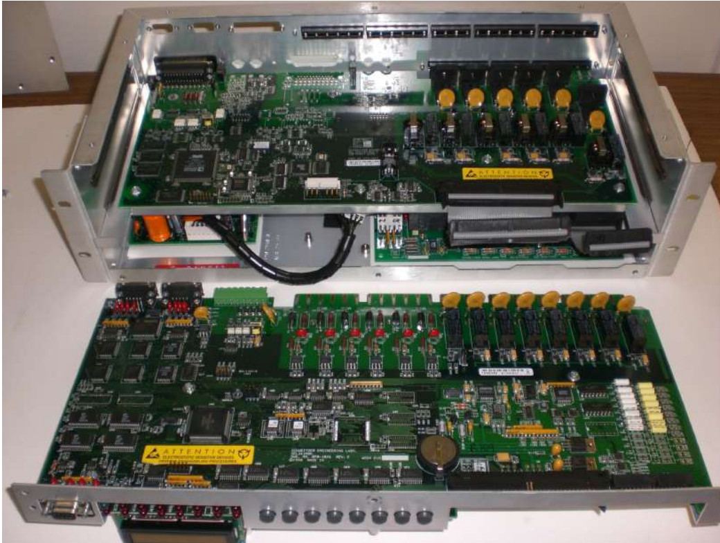
Figure 7-11. Inside the SEL-311L electronic relay unit.
