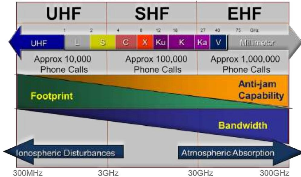
Figure 18. Satellite Communication Frequency Bands, from [26].
