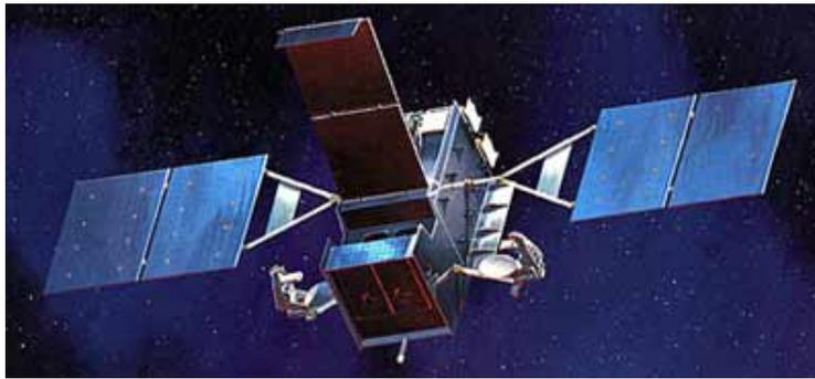
Figure 4. Space-Based Infrared System (SBIRS) Geosynchronous (GEO) Satellite, from [7].
