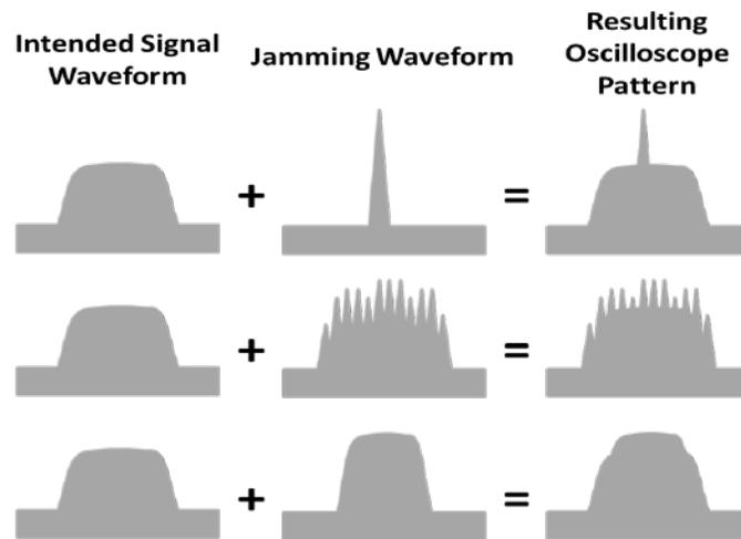
Figure 23. Example of Oscilloscope Readout with Interference, after [24].
