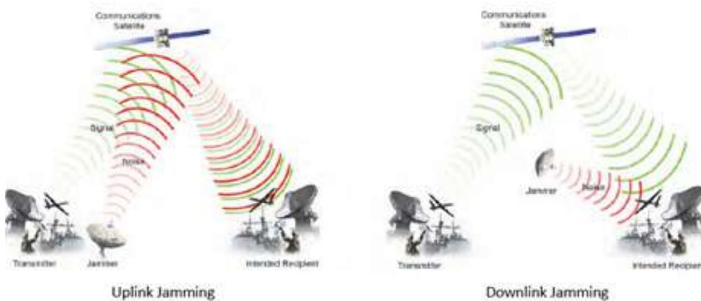
Figure 16. Examples of Uplink and Downlink Jamming, from [25].
