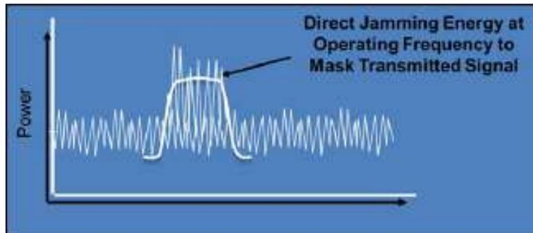
Figure 12. An Example of a Jammed Signal, from [24].
