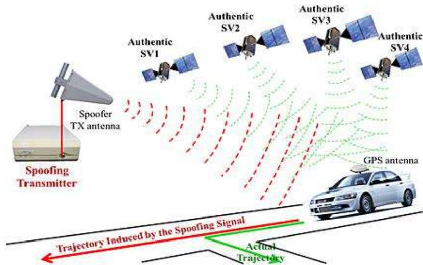
Figure 17. Effects of Spoofing on Navigation Systems, from [26].
