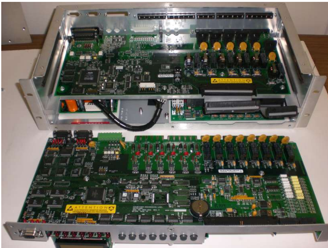
Figure 5-4. Inside the SEL-311L electronic relay unit.
