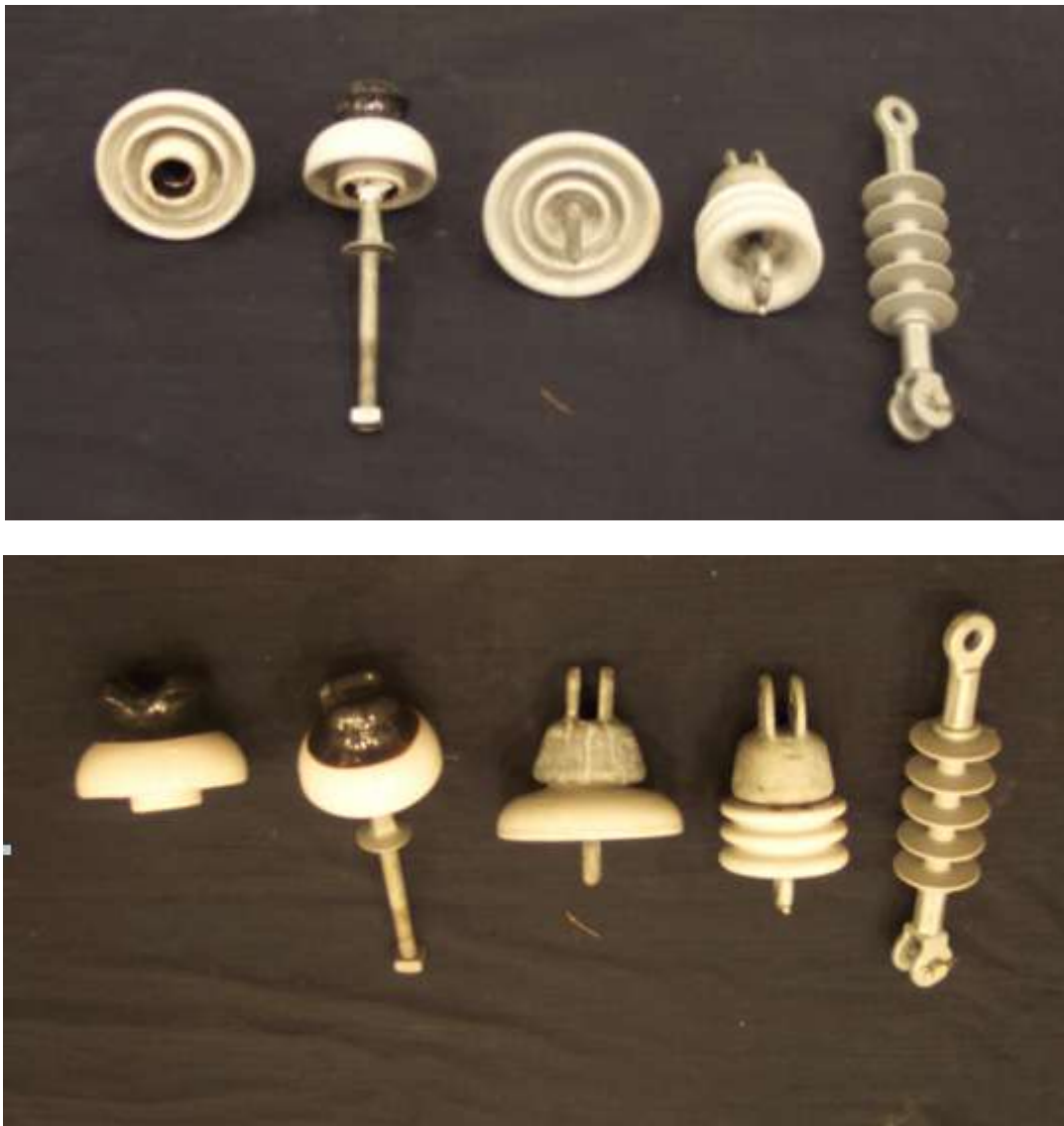
Figure 7-25. Insulators tested. This has two views of tested insulators, from the left: Pin type: ANSI 55-4, ANSI 55-3; Suspension type: ANSI 52-1, ANSI 52-9; 15 kV Polymer.
