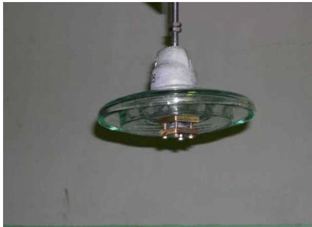
Figure 7-26. Suspension glass insulator for 10 kV power line.
