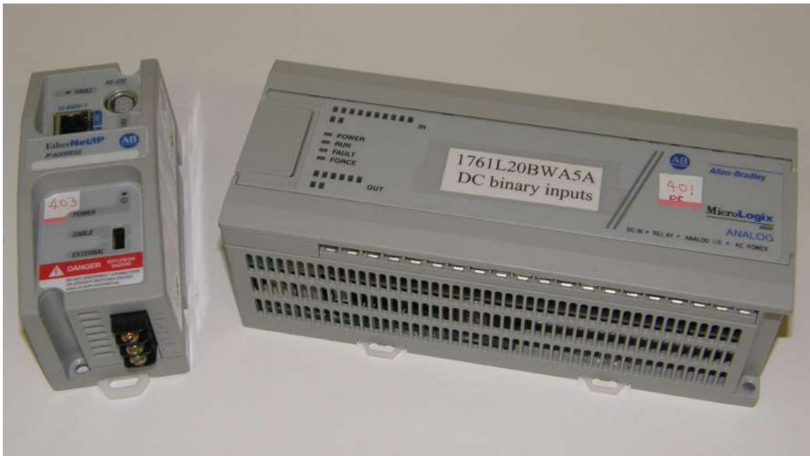
Figure 7-15. The Allen-Bradley MicroLogix 1000 PLC. The PLC, the unit on the right, has analog and binary I/O ports. Its communications is handled by the 1761-NET-ENI unit shown on the left.
