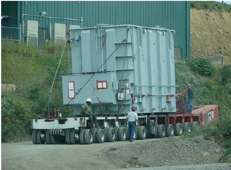
Figure 3.A.6 Shipment of One of the Largest Transformers Manufactured by ABB
