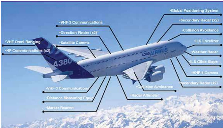
Figure 1.7. Airbus A-380 electronic systems. (Source: FAA.)
