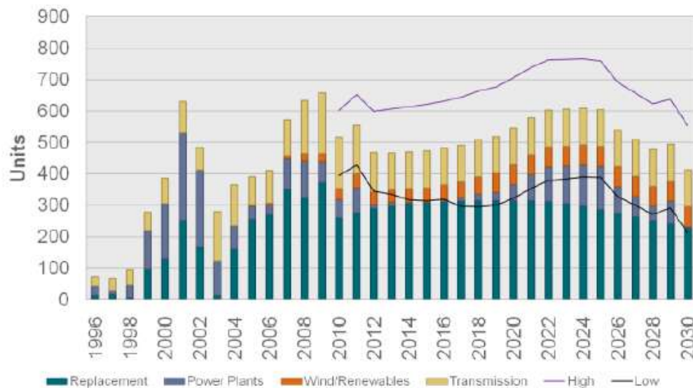
Figure 17. Projected Demand Growth for Large Power Transformers in the United States through 2030 (Power transformers with a capacity rating greater than or equal to 100 MVA)
