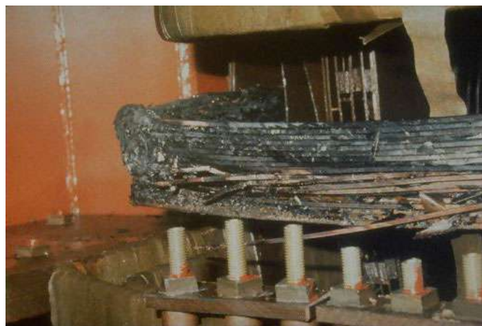
Permanent damage to the Salem New Jersey Nuclear Plant GSU Transformer caused by the severe geomagnetic storm of March 13, 1989 (Credit: PSE&G).
