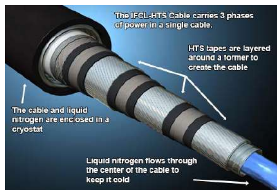
Structure of the cable (Credit: American Superconductor Corporation).
