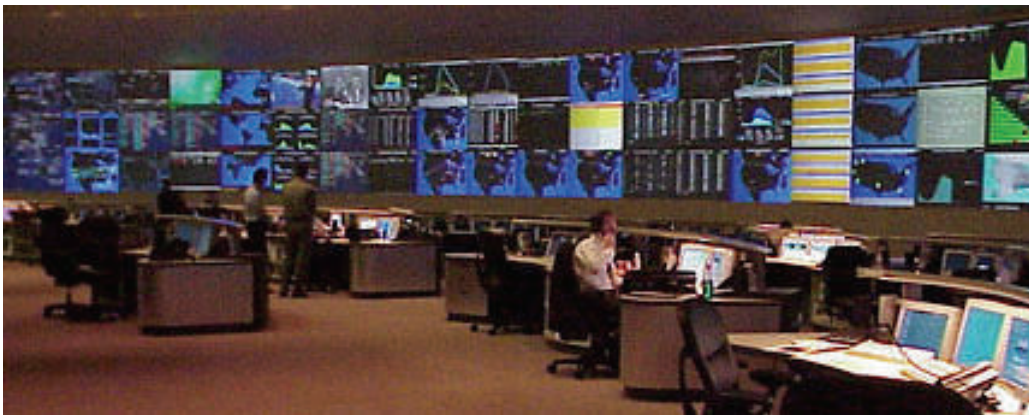
Figure 3-3. Example Network Management Facility
