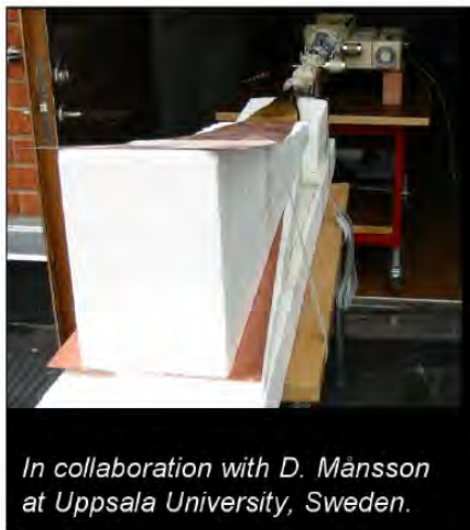
Figure 19. RADAN 303B hyperband generator used in Sweden
