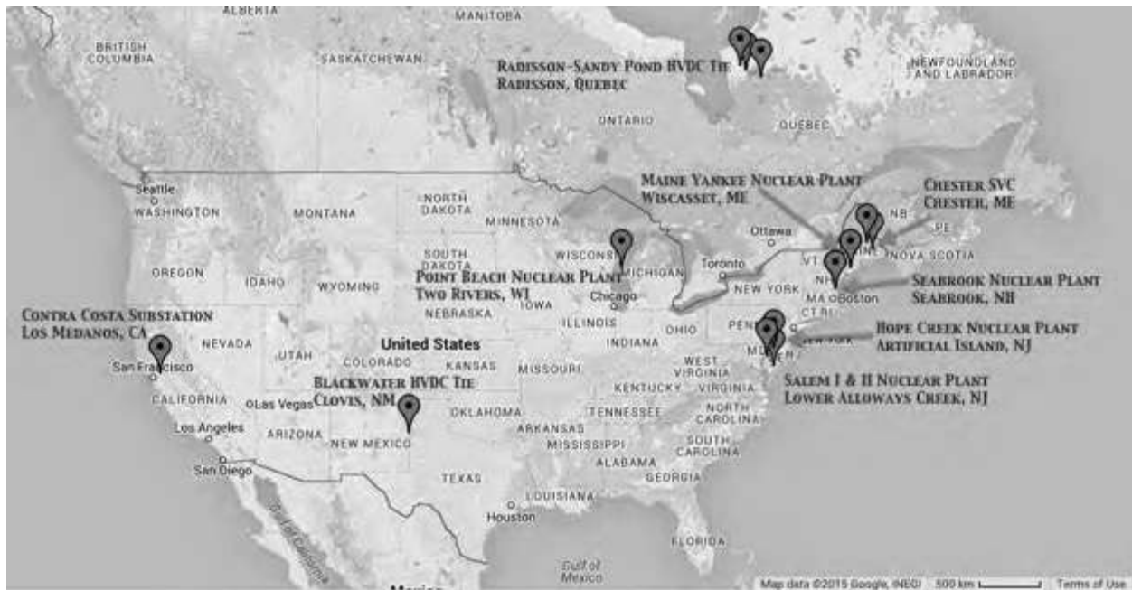
Figure 3: Select Locations of GMD Impacts on Electric Grid Facilities
