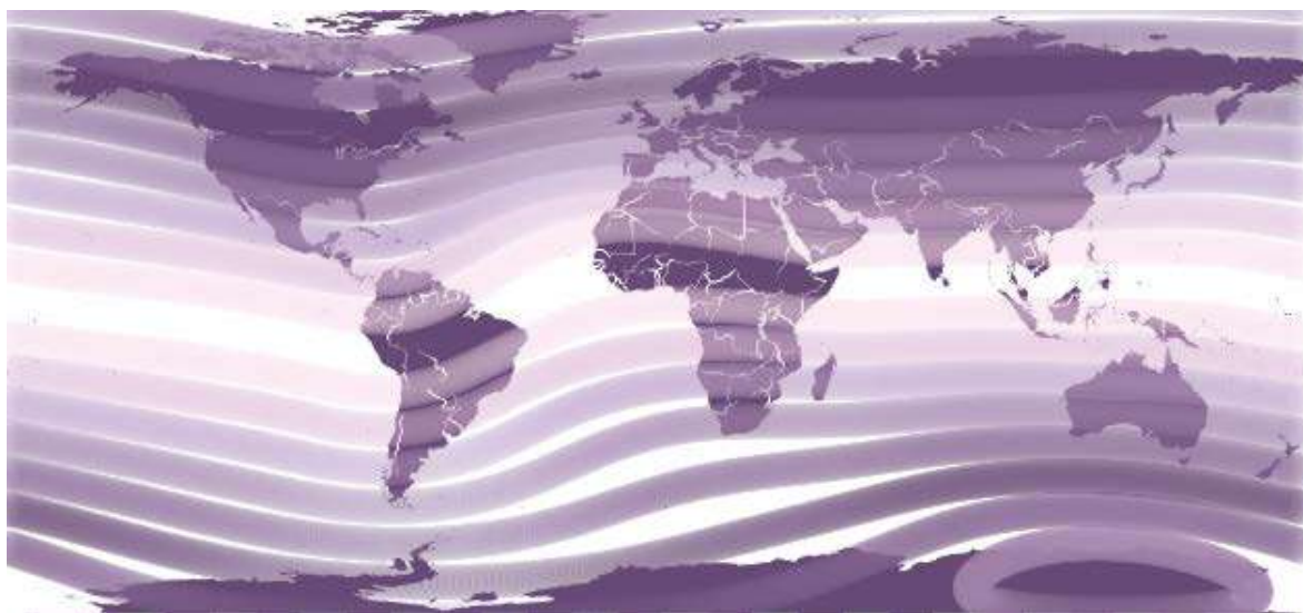
Figure 2: Bands of magnetic latitude are color-coded by AER’s model of relative risk from extreme geomagnetic storms. Dark and light purple represent regions of highest and lowest risk, respectively.
