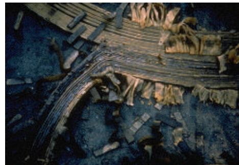
Figure 2-3. GIC Damage to Transformer During 1989 Geomagnetic Storm
